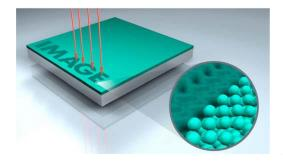
With ThermoFuse, the heat of the laser melts latex particles to form a durable image in a single step.
