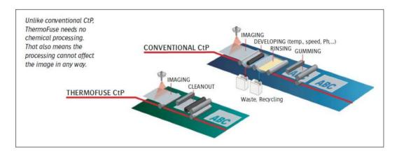
ThermoFuse imaging, unlike conventional CtP, does not rely on adapted analog processes. Using the high power of today's lasers, ultrafine thermoplastic particles are melted and fused together to create a durable image on the aluminum plate substrate in one single, digital step.
